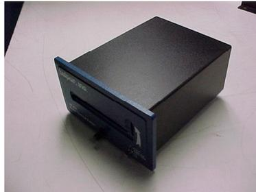
Remove cover by rotating the latch counter-clockwise until the latch disengages from the cover.
