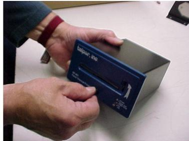
Once latch disengages the cover will slide out easily.
