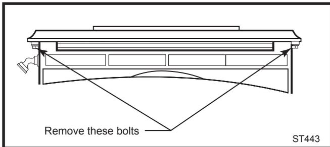
**Fig. 31** Remove four bolts securing stove top plate.
