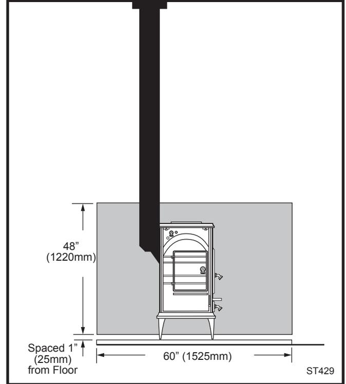
Fig. 17 Sidewall protection.
