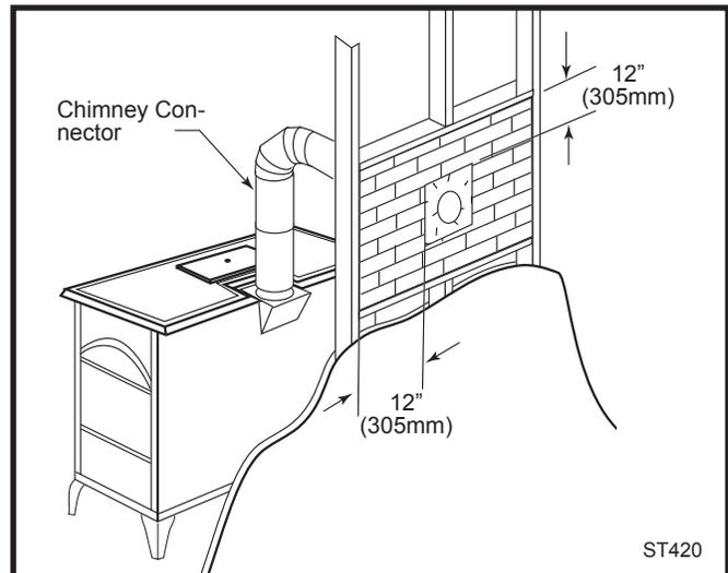
Fig. 10 Wall pass-through enclosed with noncombustible materials.
