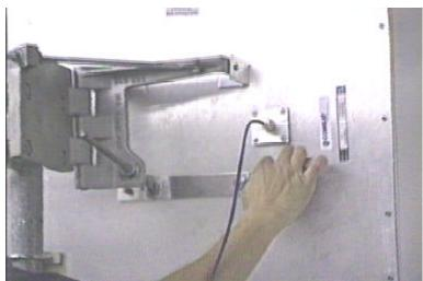
All Solectek antennas are set to vertical polarity at the factory. To change the polarity, locate the four small bolts on the back of the antenna which fasten the antenna to the mounting bracket (either Standard or Universal mount).
