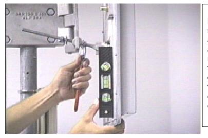
Use a bubble level (carpenter's level) to make sure the antenna is set to a vertical position prior to attempting the initial antenna alignment. It is usually not necessary or desirable to change this adjustment for normal operation. Note the use of the wrench on the threaded rod to change and lock/unlock the elevation adjustment.
