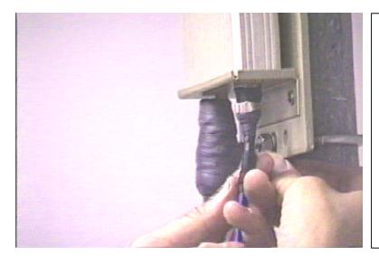
Stretch the black sealant material while wrapping it around the connector. It should be possible to get a good seal on this small (TNC-type) connector with only one sealant strip. If necessary, use a second strip to ensure a weather-tight seal.
