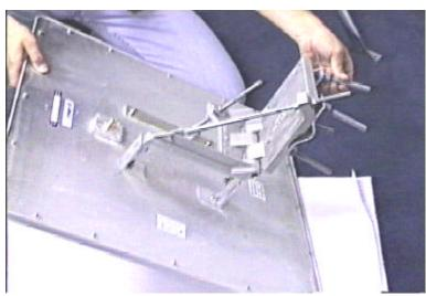
This is the optional "Universal Mount". This mount uses threaded rods to adjust the azimuth and elevation once the antenna is permanently mounted on the mast. Preassemble the mount before attempting to mount it on the mast. This mount uses the same mast straps and mounting bolt as the "Standard Mount'.
