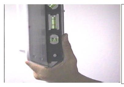
Use a bubble level (carpenter's level) to make sure the antenna is set to the vertical position before attempting the initial antenna alignment. It is usually not necessary or desirable to change this adjustment for normal operation.
