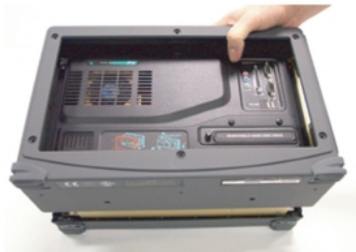
Figure 5.2 Remove the Outer Casing
