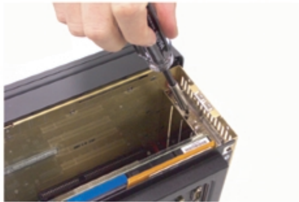
Figure 5. 6 Expansion Slot Cover - Single Screw Removal
