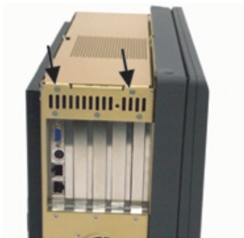
Figure 5. 4 Two Card Retention Plate Screws
