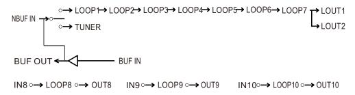
Guitar signal feeds into OC10 input (NBUF IN or BUF IN), enters series LOOP1~LOOP7 when MUTE switch is off, then outputs from OUT-1 and OUT-2. when TUNER switch is pushed, the signal outputs to TUNER jack. Be noted the BUF OUT jack doesn't output when the guitar plug into NBUF IN jack.
