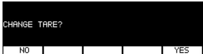
The Tare ID# exists but you can bail out of changing it by pressing the **NO** soft key. The display returns to the **Edit** screen. If you press **YES** the following is displayed:
