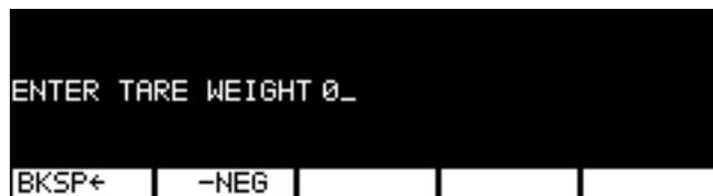
Key in the tare weight and press the **ENTER** key. The **Edit** screen returns. Go to step 10.
