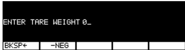
Key in the tare weight and press the **ENTER** key. The opening screen returns in net mode with the tare active.
