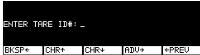
5. Key in a tare ID number to identify this tare and press the **ENTER** key. See note on step 4.
