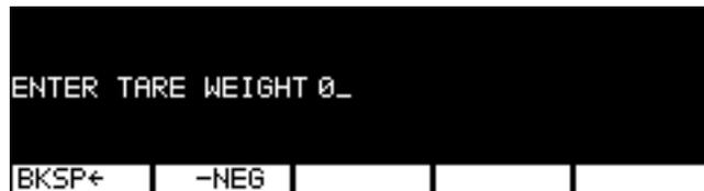
Key in the tare weight and press the **ENTER** key. The **Edit** screen returns.
