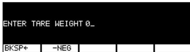
Key in the tare weight and press the **ENTER** key. The following screen is displayed.
