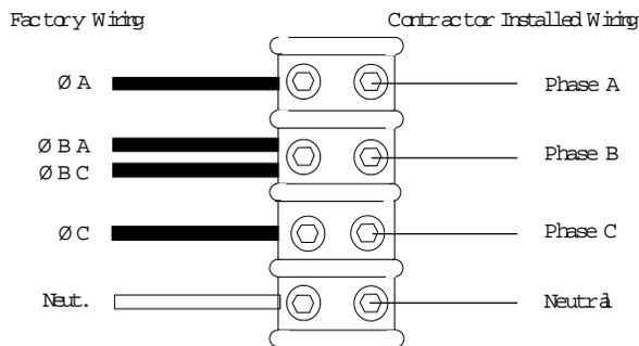
Double-check all connections, and make sure all terminals are tightly secured before replacing cover. Tighten the cable clamp and connect the cable to a suitable power source.
