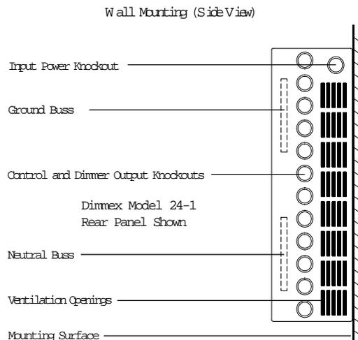
If common load neutrals absolutely must be run (retrofit situations), do not connect circuits of the same phase to the same common neutral wire. Do not run more than three dimmers (three-phase) or two dimmers (single-phase) on a common neutral wire. Choose the size of the neutral wire to handle 120% of the rated dimmer load.
