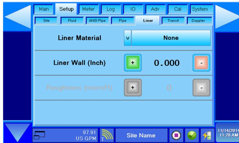
Figure 10: Liner setup
