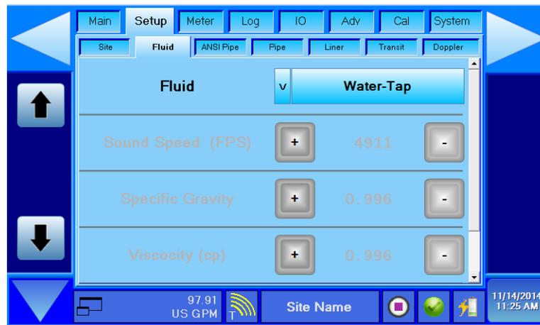
Figure 7: Fluid setup
