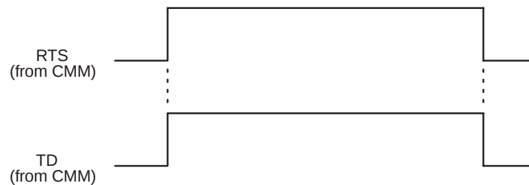
Figure 2-7. Flow Control = NONE, MODEM TURNAROUND DELAY=0
