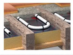
IN JOIST FOIL BOARDS
