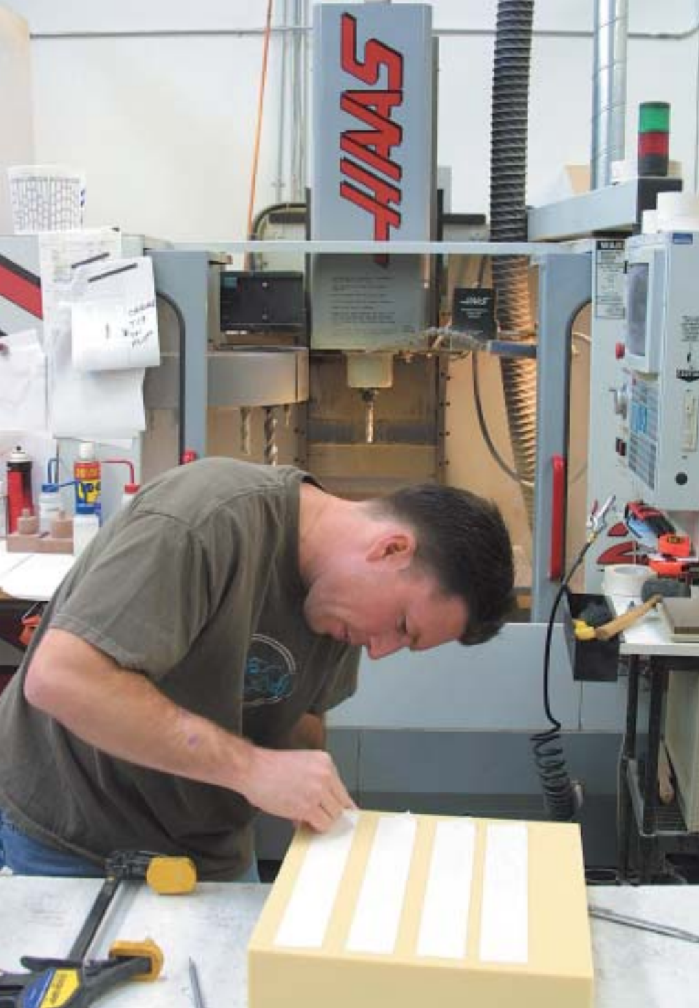
Industrial designer Bill Debley (left) uses double-sided tape to secure a piece of foam for machining, while a VF-8 (top) cuts plastic for a prototype as an air gun keeps things cool.
