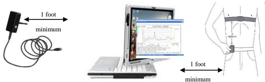
Short range receiver (no antenna) **must be at least 1 foot away the computer.** Long range receiver (with antenna) may touch computer.
