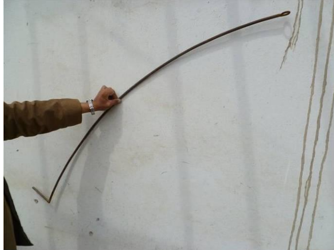
Photo 8.3: Arch Guide. Loop at Right End for Pivot on Vertical Central Pipe.
