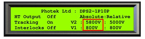
The voltages displayed here are the actual voltages applied to each electrode. These are the absolute values that would be measured referenced to ground (0V).
