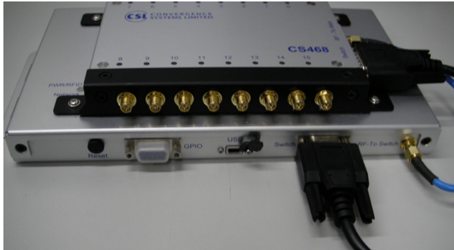
Figure 4-2 CS468 Reader Side View
