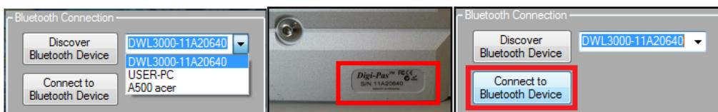
8. When the connection is established successfully, all function toolbar buttons are turned on and the status bar shows "Device Connected and DigiPas® Security Dongle is found". The DWL3500XY PC Sync is now connected to the Device and ready for use.
