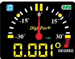
4. Bluetooth logo appears on the device screen (at top-right corner). The device setting is now completed. User can proceed to synchronise the DWL3500XY device with the PC Sync software.
