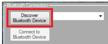
7. Bluetooth devices is shown at the drop down box. Select the device with the serial number indicated as shown on the drop down box and press "Connect to Bluetooth Device button" to establish the wireless connection.
