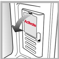
**ODOUR FILTER\***: some models are fitted with a new active carbon odour filter, which ensures better air quality inside the refrigerator. The filter is located on the bottom right-hand side, inside the ventilation opening. To activate it, remove the sticker from the opening (*see diagram*).
