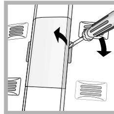
To replace the light bulb in the refrigerator compartment, disconnect the plug from the electricity mains.
