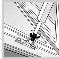
The stiffness of the door opening/closing movement for the bar compartment may be adjusted. When you are in front of the appliance, turn the two lateral rods to the left if you wish to stiffen the movement, or to the right if you wish to loosen the movement.
