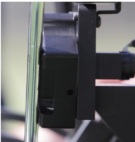
Once you reverse the drill and relieve the pressure, the shaft should be perfectly flush with the cradle. If not, bend it again until it is.
