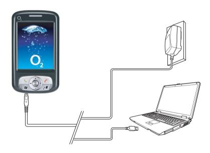
AC Adapter: Connect the battery charger to a suitable main power socket and the charger plug into the connector of your Xda Atom. Note on the orientation when plug in.  USB Cable: Connect your Xda Atom to your PC's USB port with the USB cable supplied in your package as shown above.
