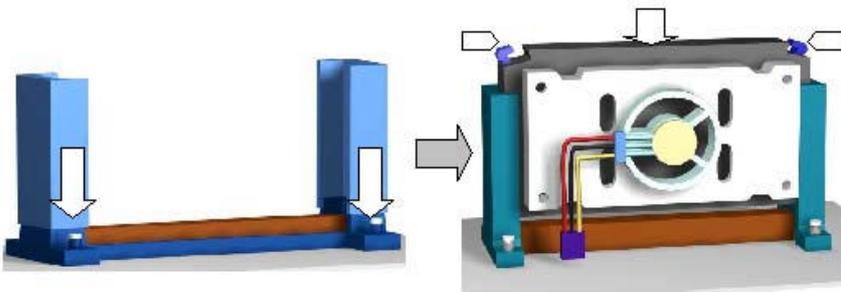
3. Push 4 lock pins into holes to fix Retention Mechanism on motherboard.
