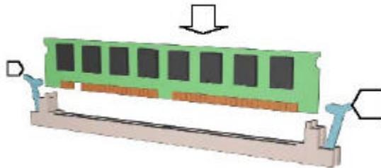
Be careful not to misfit the DIMM Module into DIMM sockets in wrong direction. This module can be inserted into the socket only one way. To release the memory module, push both latches down and carefully rock the module forward and backward while slowly lifting it upward.
