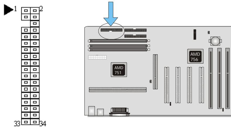
The FDC sub-system can control three types of floppy drives (1.2, 1.44 and 2.88MB) or compatible tape drives. The connection to the floppy drive is via a header. The floppy disk interface includes 48mA drivers and inputs on the drive interface.
