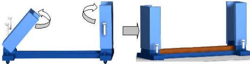
1. Unfold the Retention Mechanism.
