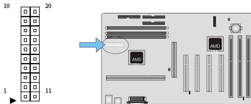
This connector supports a standard ATX power supply. When connecting, make sure the lock key matches the hook attached on a power supply cable. The power cord should be unplugged when you connect it.
