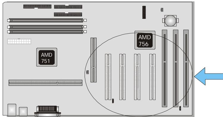
This motherboard contains 8 expansion slots (including one shared PCI/ISA) onboard. Three 16-bit ISA Bus, four 32-bit PCI expansion slots and one 32-bit AGP slot are shown as above.
