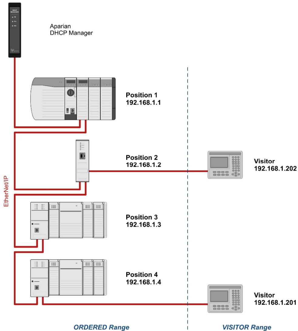
Figure 1.2. - Example of a network setup in Normal mode
