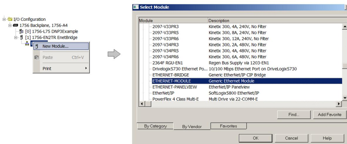
Figure 3.24 - Add a Generic Ethernet Module in RSLogix 5000
