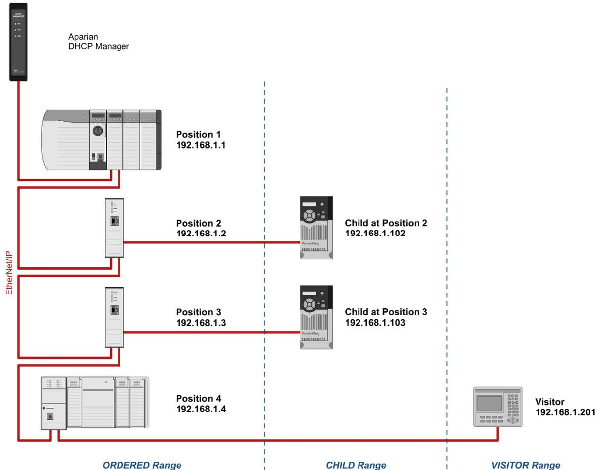
Figure 1.3 – Example setup of network in ETAP-Child Mode
