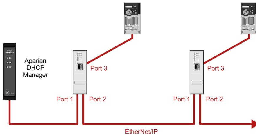
Figure 1.4 - Three-port device connection – Must enter on Port 1
