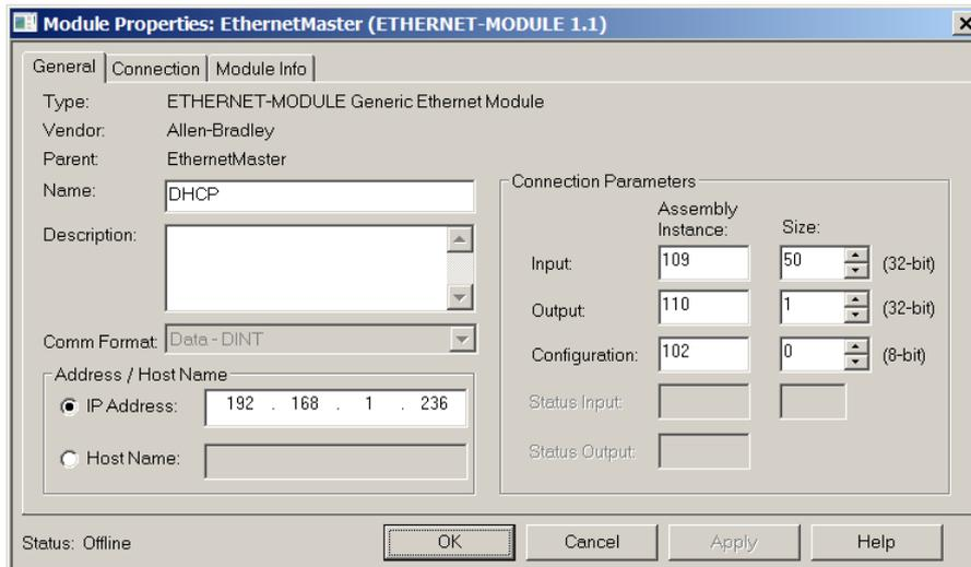
Figure 3.25 - RSLogix General module properties in RSLogix 5000
