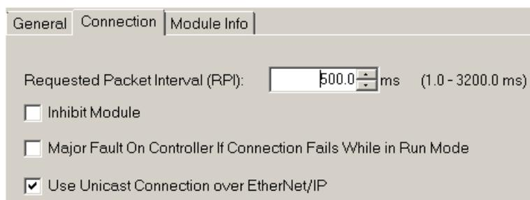
Figure 3.26 - Connection module properties in RSLogix 5000
