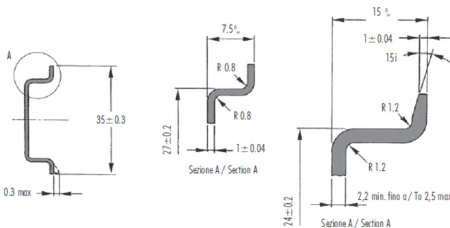
Figure 9.6.2 - Required DIN dimensions
