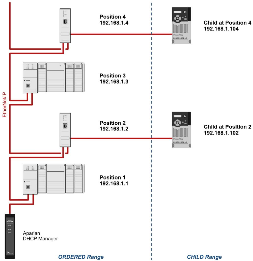
Figure 1.5 - Example setup of network in ETAP-Child Mode
