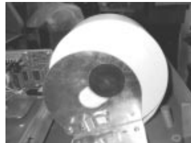
Figure 6-3B The Paper Spool in position for removal.
