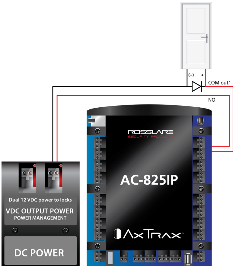
Figure 3: Door Lock – Failed Close
