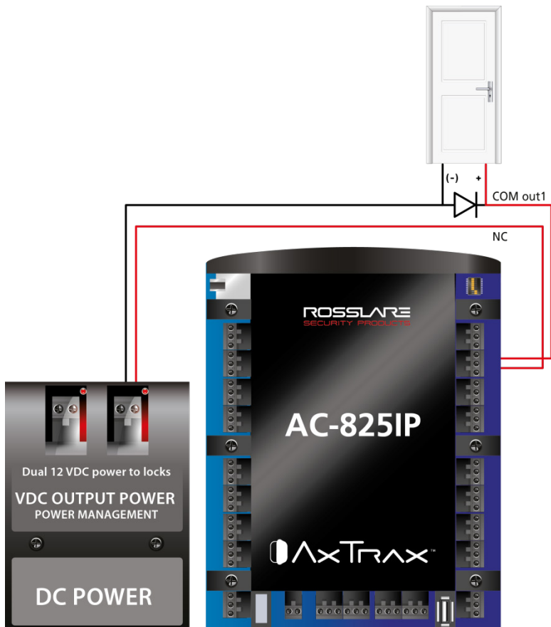
Figure 4: Door Lock – Failed Open
