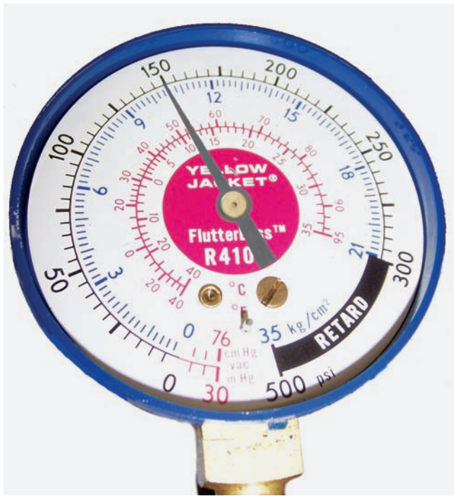
Figure 25-38 This gauge is reading 150 psig with a saturation temperature of 45°F for R-410a
