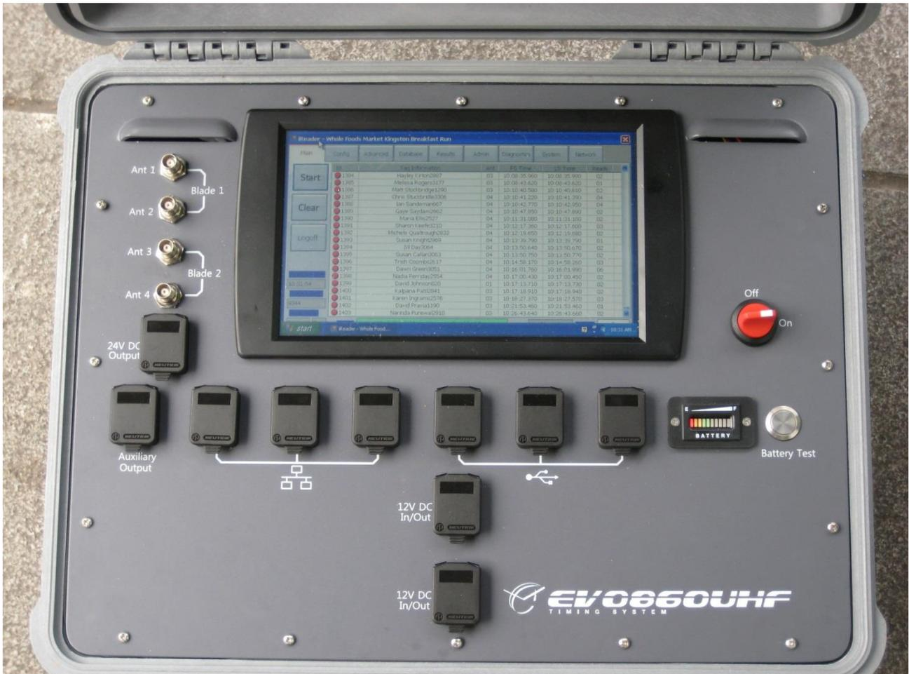
The Mk2 unit is housed in the same Peli case but has a very different main panel layout. The Mk2 uses a new controller PC which adds additional functionality with dual wired network connections allowing the internal reader to be isolated from the main network and comes with WiFi as a connection option. The basic Mk2 is a four-port unit like the Mk1 – the two variants use the same internal tag reader.
