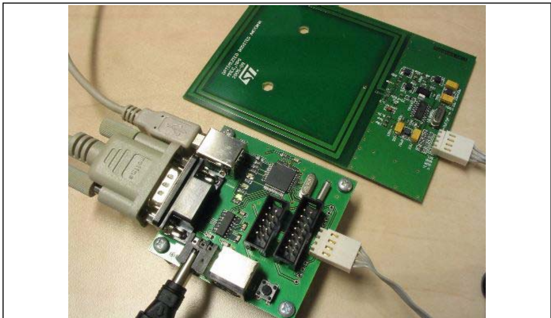
Figure 1. Demokit hardware for a short-range RFID reader with autonomous functions
