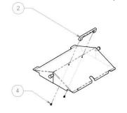
Figure 3. Bath Cover Assembly Step 1
