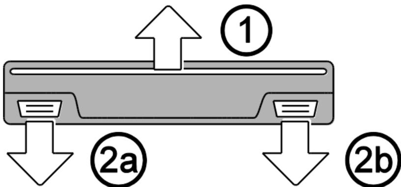
2. The unit is spring loaded and opens to its full reading position. If the unit is off, it automatically turns on when the reading stand opens.
