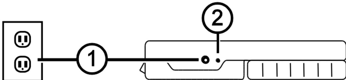
2. The battery indicator LED blinks green to show that the battery is charging (2).
