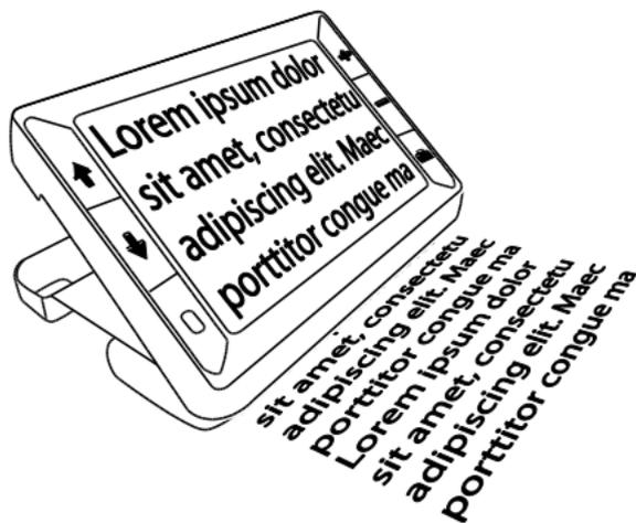
4. When you close the reading stand, the unit automatically turns off.
