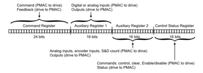
As messages are passed around the ring, each slave device evaluates the message to determine if the message is addressed to that slave. If either the master or slave identifier contained in the message does not match the slave's ID values, the message will be passed to the next node on the ring with no modification. If both the master and slave ID values match the slave, the slave will pass a response message to the next device on the network.
