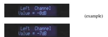
Here you can change the balance setting by reducing the gain of the left signal source. By pressing the volume keys the amplification can be changed in steps of 1dB.
