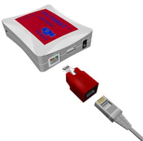
Connect the crossover module to the LAN cable of the camera. Connect the crossover module to the USB Driver (Connection 1 in Device Description).
