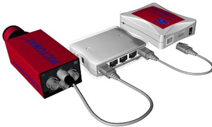
Connect the LAN cable of the camera to the switch. Connect the USB Driver to the switch using the LAN cable (Connection 1 in Device Description).
