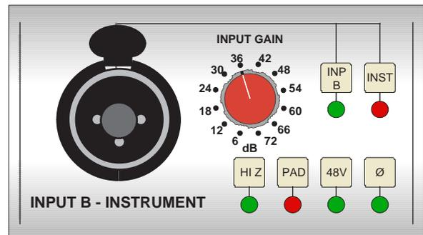
The stepped **INPUT GAIN** control has a gain range of +6dB to +72dB in 6dB steps.
