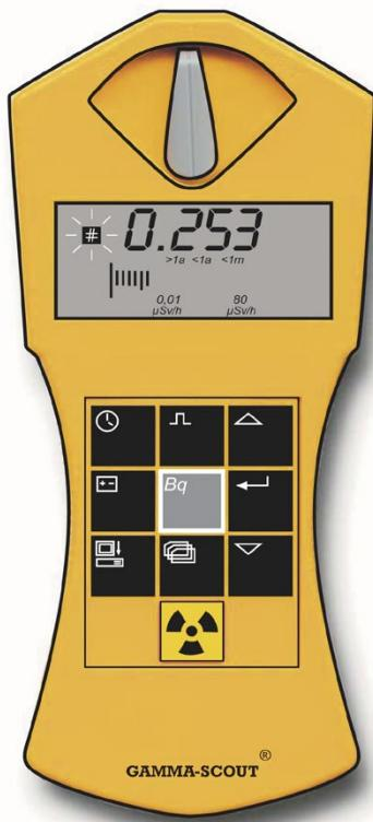
GAMMA-SCOUT® has an integrated quartz clock whose display you can activate by pushbutton. Time and date are used to register the measured radiation. The PC-supported software has a feature to synchronize the GAMMA-SCOUT® date and time with your PC-clock. The GAMMA-SCOUT® clock serves to file data.
