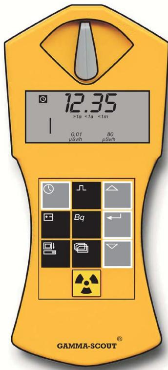
GAMMA-SCOUT® is powered by a Lithium/Thionyl chloride cell of 2.7 - 3.7 voltage. The device will continue functioning until the cell voltage is down to 2.7. When the voltage drops below this value, the battery symbol will appear in the display. The stored data should then be read from the internal memory. Nevertheless, the data will be retained even at total breakdown of voltage, and can then be read when the device is serviced. Indicating the battery voltage
