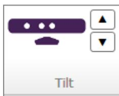
You can adjust the up-down direction of the Kinect using this function. Please do not use your hand to directly move Kinect up or down, as it could cause fault.
