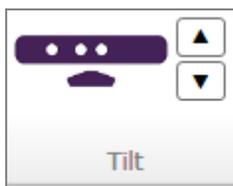
You can adjust the up-down direction of the Kinect using this function. Please do not use your hand to directly move Kinect up or down, as it could cause fault.
