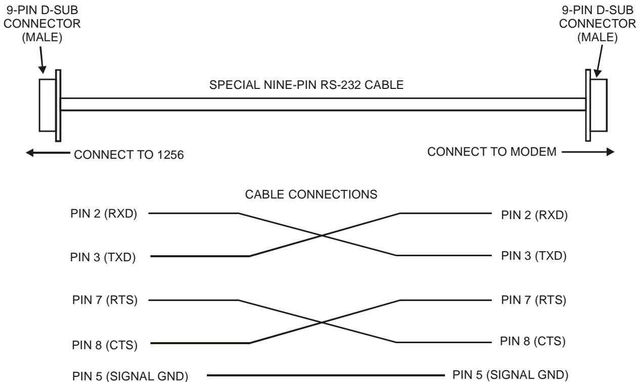
Figure 4-4b, Using the 1256 with a Modem
