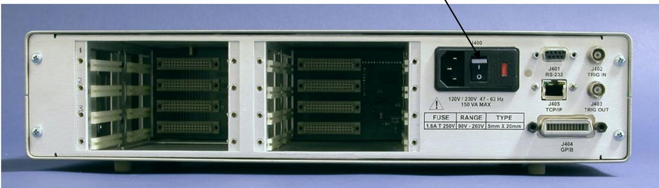
Figure 2-4, Activating Main AC Power
