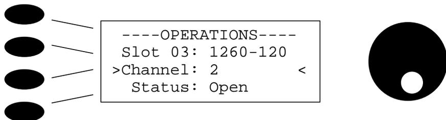
Line 4 shows the status of the channel 2 relay on the 1260-120 plug-in.
