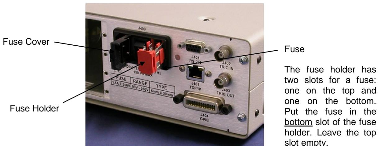
**Figure 2-1, Changing Fuse for Main AC Power**
