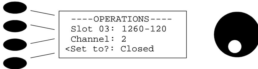
On the fourth line, the 1256 asks whether to close the relay channel:
