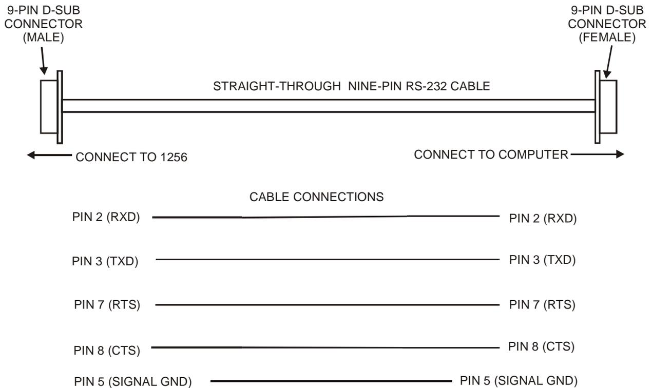
Figure 4-4a, Using the 1256 with a Computer
