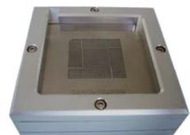
4. Lock the fixed slider of the two no-spring slider, take out the BGA chip and wipe a layer of solder paste, fixed the chip on the adjustable reballing kit again, cover the cap.
