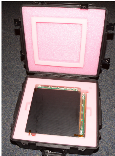
Figure 26. Ionization chamber in shipping case with protective window covers fitted
