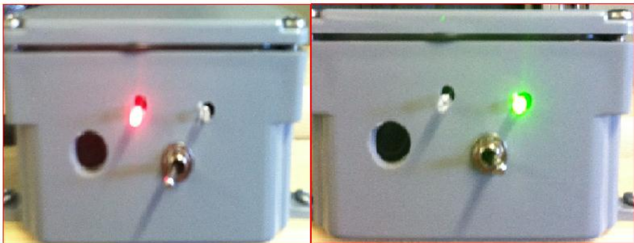
Figure 4.7: Left red LED and switch orientation during failure occurrence, Right green LED and switch orientation during system restorance
