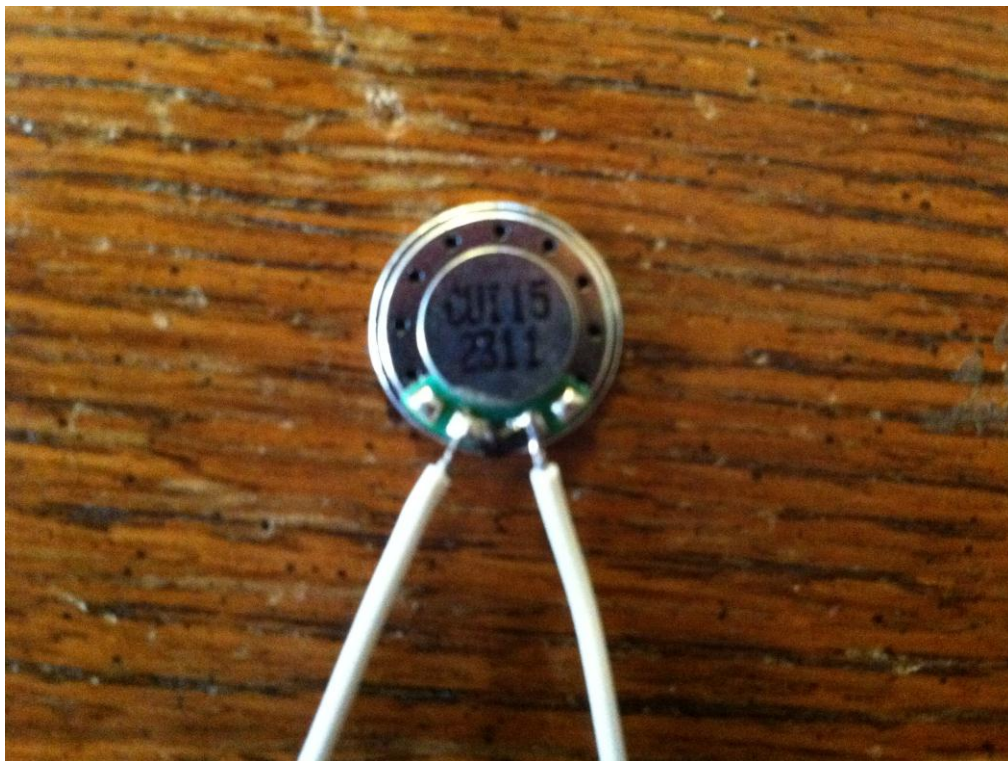
Figure 2.2.2: Leads Connected to Speaker
