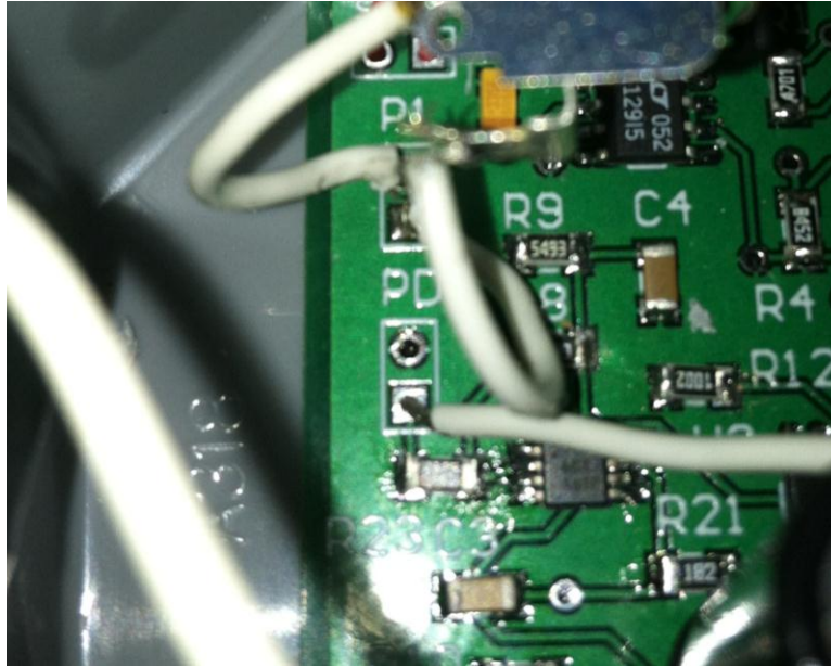
Figure 2.2.7: Photodiode Connection on Board
