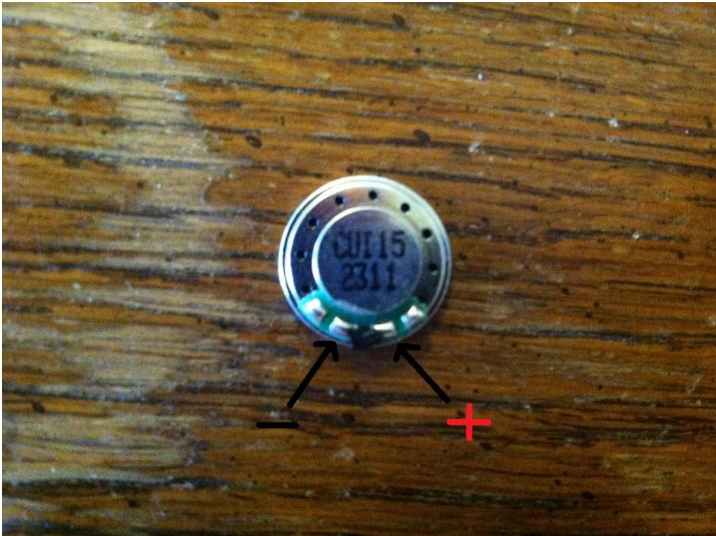
Figure 2.2.1: Polarity of Speaker
