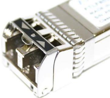
**Figure 14a:** SFP+ latch closed
