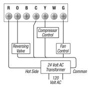
**NOTE:** For reversing valve active in heating, use B terminal instead of 0.
