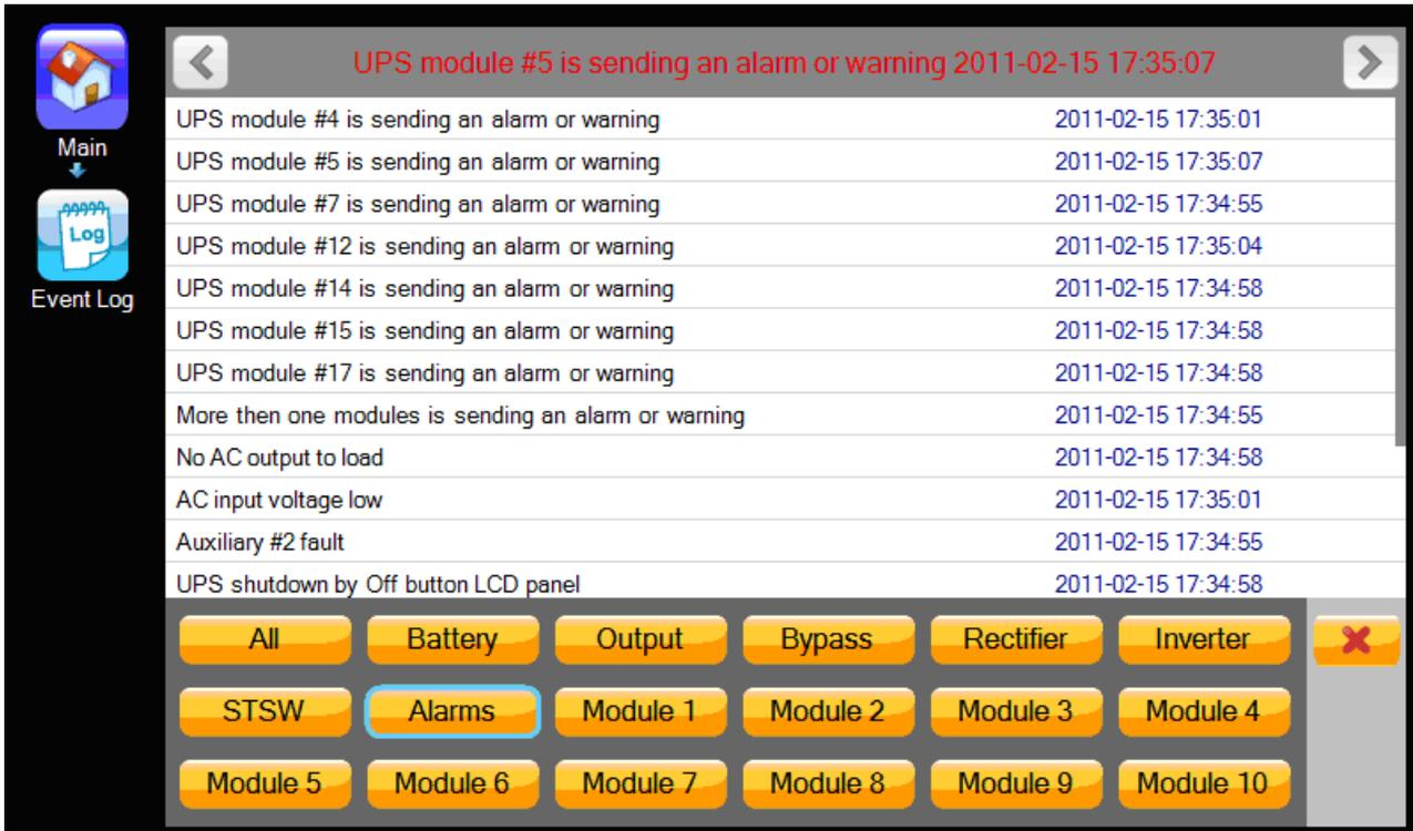
Figure 52: "Alarms" display from the log detail screen
