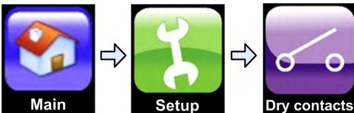
The Dry Contact function under the Setup option assigns alarm conditions to the output dry contacts. When the specified alarm occurs, the contact closes. The output dry contacts can be used to trigger external devices. See section 6.1.9 for details.
