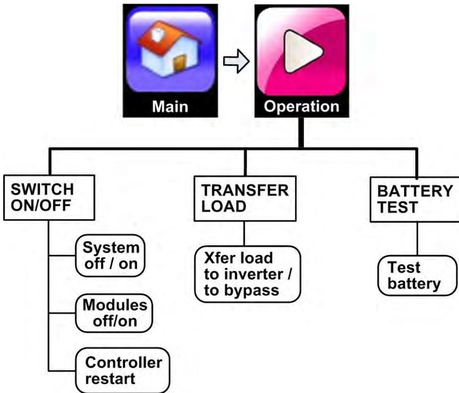
Figure 45: The "Operation" option on the main menu
