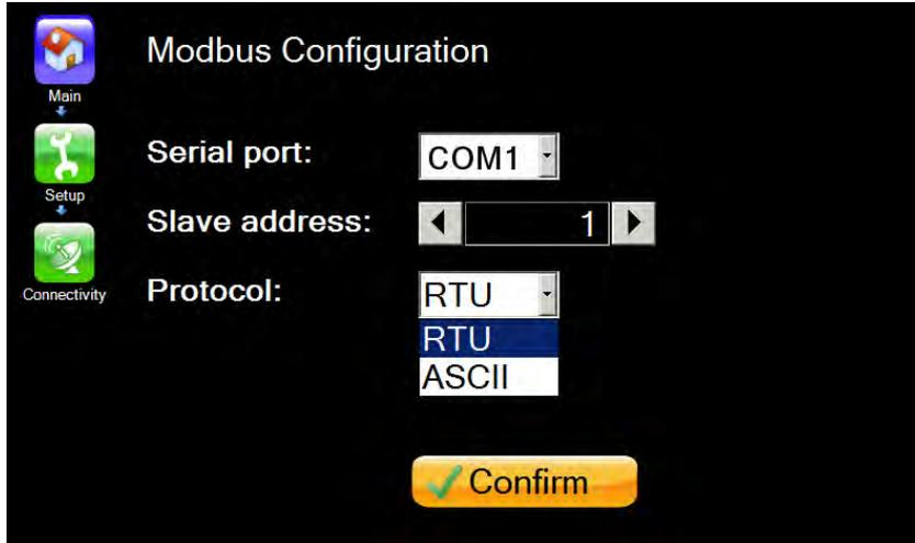
Figure 25: Defining Modbus communication parameters
