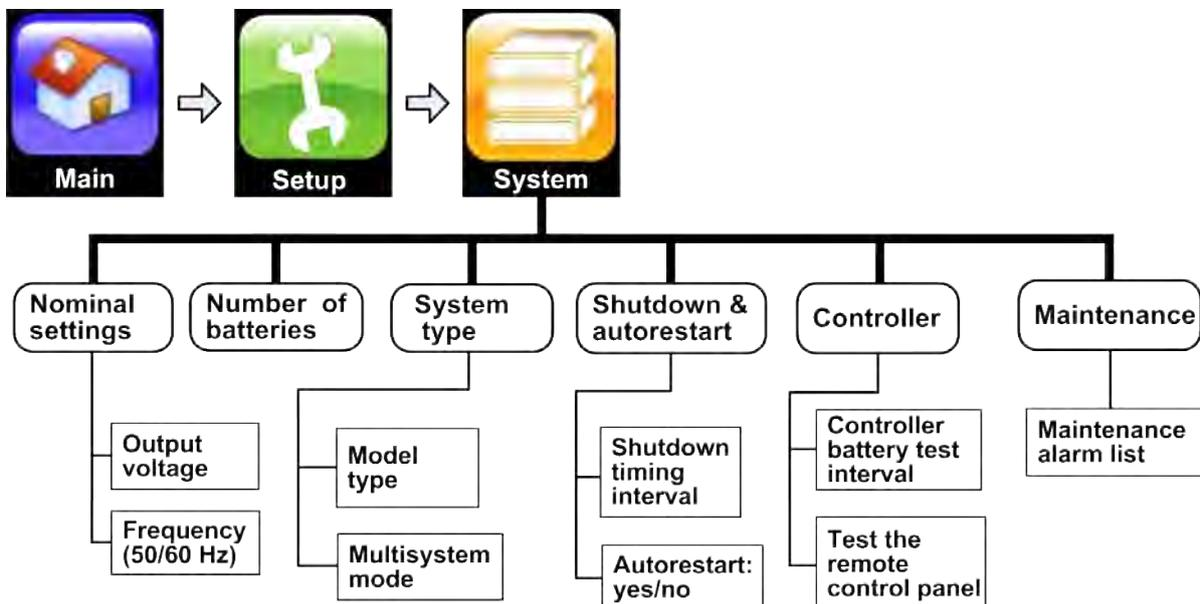
Figure 15: "Setup > SYSTEM" options
