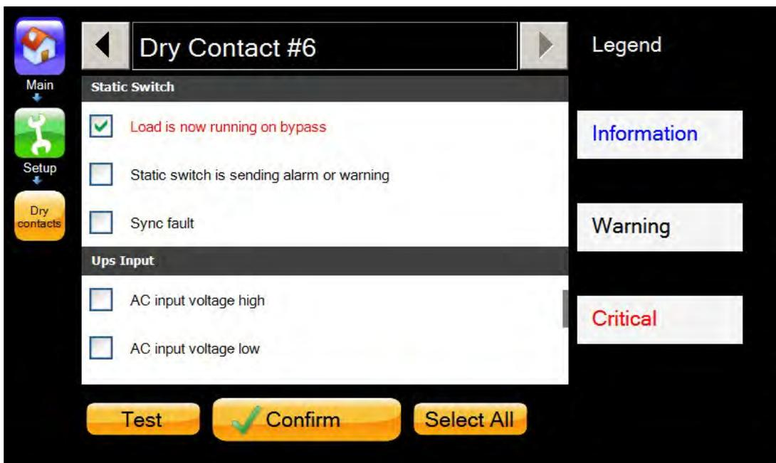
*Figure 41: Example of an output dry contact linked to an alarm*
