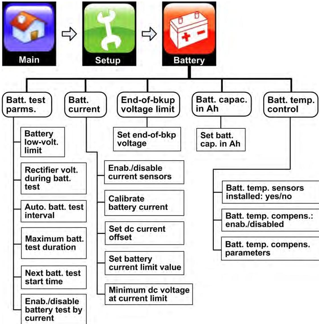
Figure 17: "Setup > Battery" options
