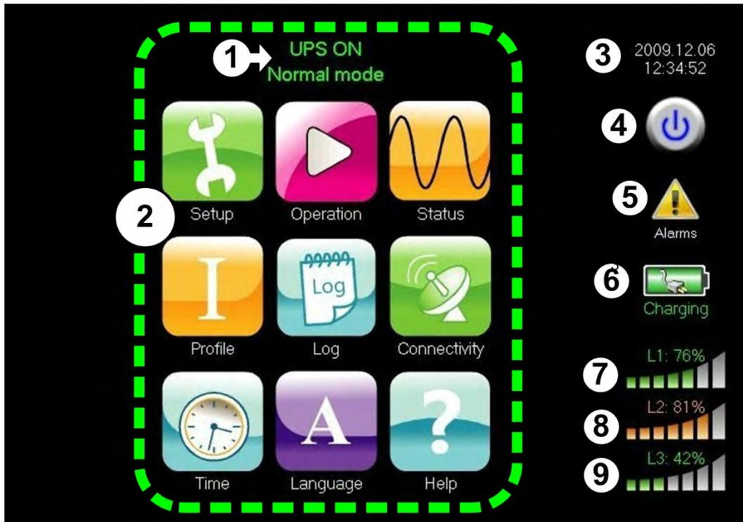
Figure 5: The main screen and its features
