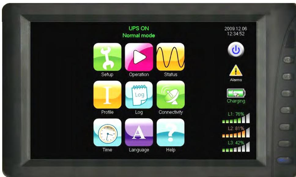
**Figure 4: The control panel**
