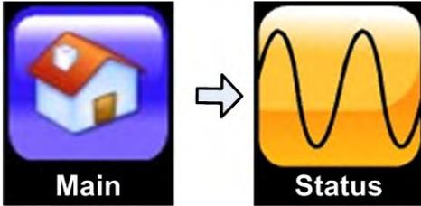
Selecting the Status option on the Main Menu displays a diagram that summarizes the overall state of the UPS.
