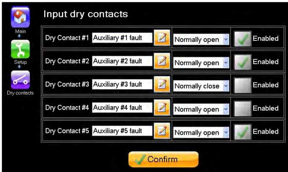
Figure 40: Defining an input dry contact
