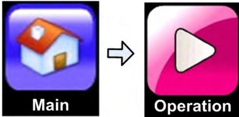
The Operation option on the Main Menu is used to turn the UPS on or off.
