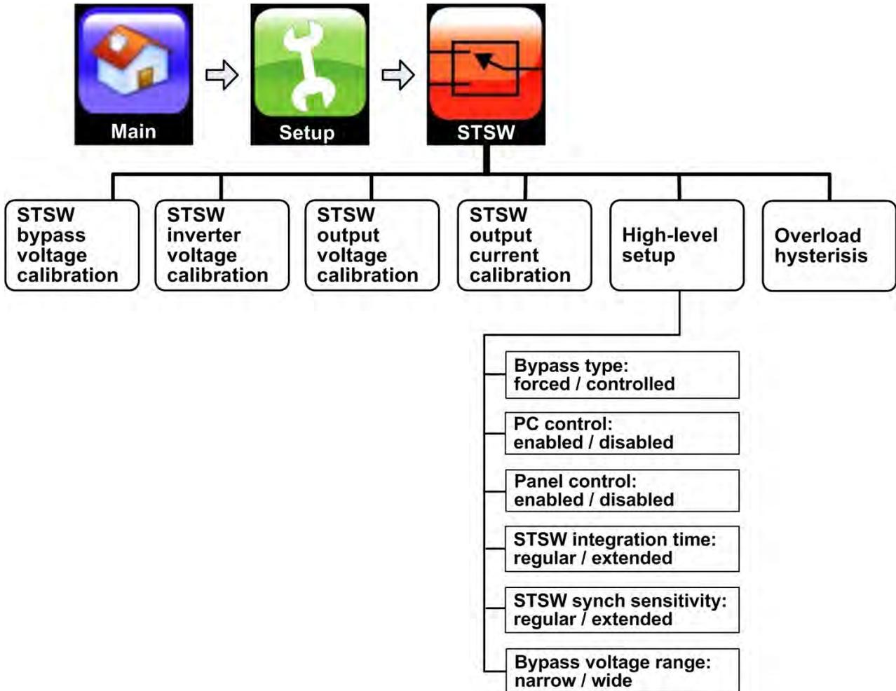
Figure 18: "Setup > Static Switch" options
