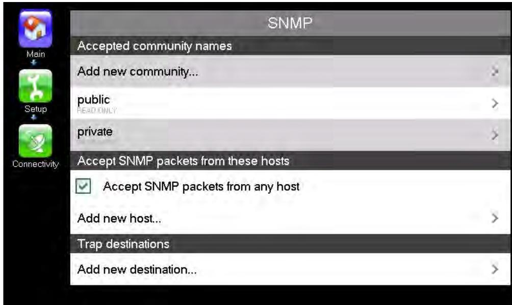
*Figure 21: Setup > Connectivity > SNMP configuration options*
