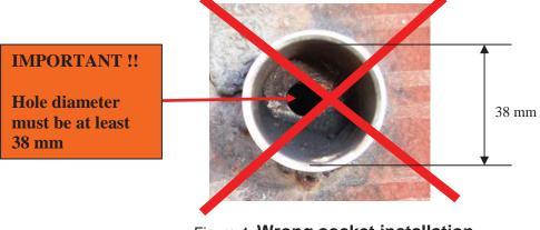
Figure 4. Wrong socket installation, THE DIAMETER OF THE HOLE MUST BE MINIMUM 38 MM
