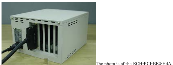
Figure 2.8. Plugging the power cable into the ECH-PCI-BE2-H4A
