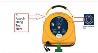
IF YOUR DEVICE LED IS RED OR UNLIT AND YOU NEED IT IN A SUDDEN CARDIAC ARREST EVENT, REPLACE THE INSTALLED PAD-PAK WITH THE RESERVE PAD-PAK PER THE INSTRUCTIONS ON THE REVERSE.
