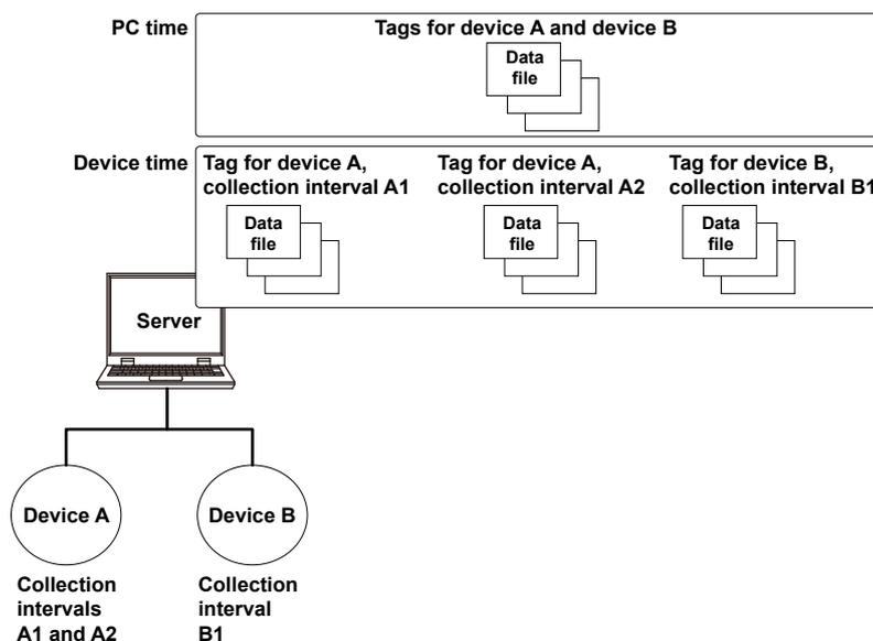
The device number, device name, and device acquisition interval are included in the names of data files. Below is the file name format when date and time are included.
