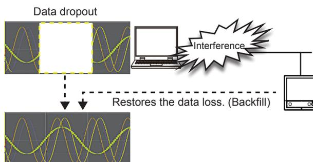
Several conditions must be met for the backfill function to operate properly. For details, see Q4 on [page 7-5](#).
