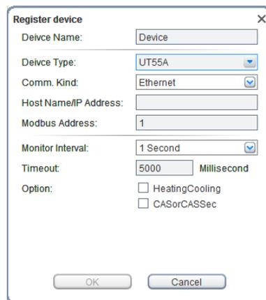
The name of the registered Modbus device appears next to Device Type in the **Register device dialog box**.\*
