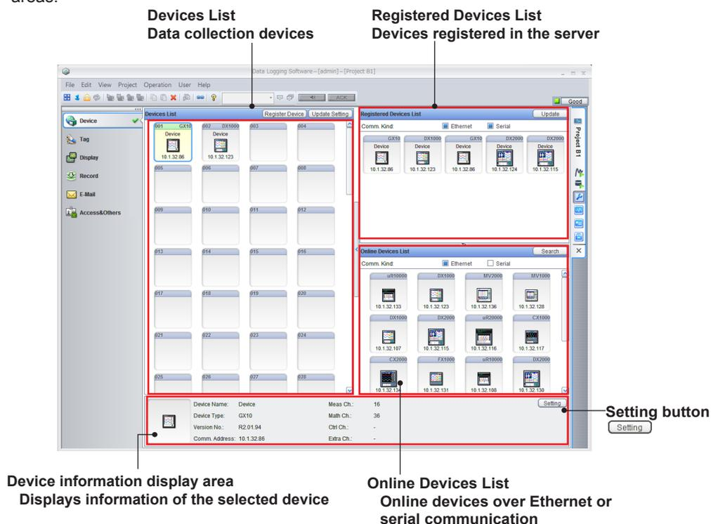
Device icons (shown in the following figure) display the devices' information. These icons are used to register and delete devices between the Devices List, Registered Devices List, and Online Devices List.
