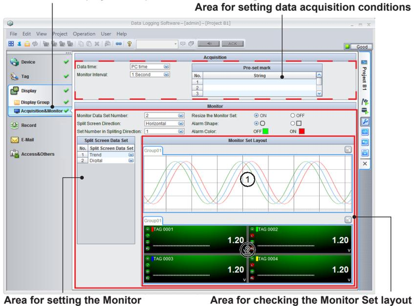
The Acquisition & Monitor Page is divided into two areas: an area for setting data collection conditions and another for configuring the monitor. The details of each are provided in the following pages. Use the letters (a to j) in the figure to reference the corresponding descriptions.
