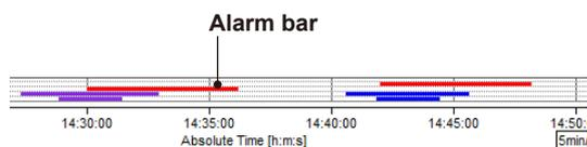
The bars show the data range in which alarms are occurring for the tags displayed in the group. The alarms are from the top alarm level 1, alarm level 2, alarm level 3, and alarm level 4.
