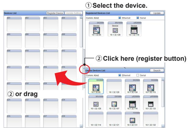
To add a device using the Register Device, follow the procedure below.
