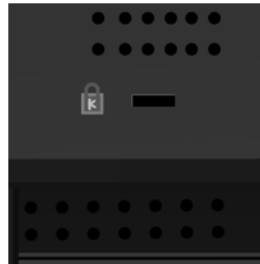
Figure 2-3 A Typical Kensington Lock
