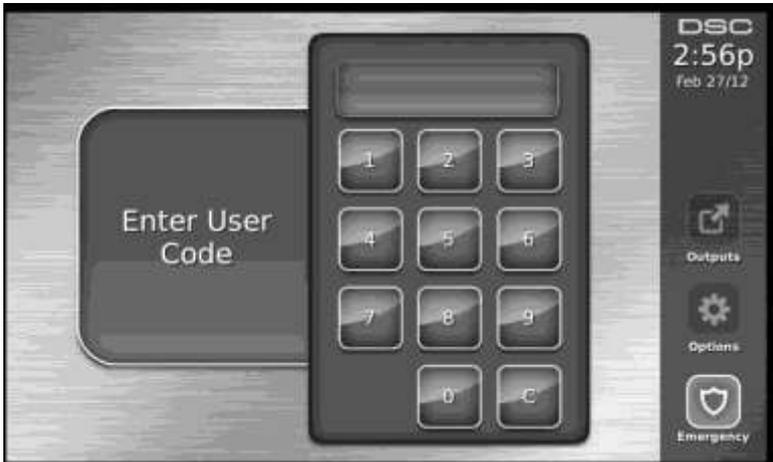
If Disarm is selected during the exit delay, a numeric keypad is displayed.
