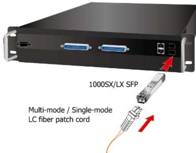
Figure 2-2-3: Plug-in the SFP transceiver
