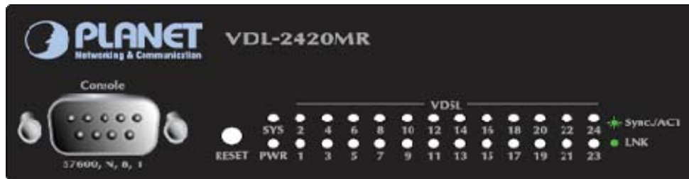
Figure 2-1-2: VDL-2420MR Series System and Port LED panel
