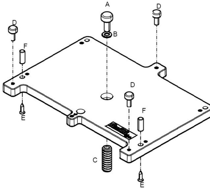
Figure 12. Installation of the base plate
