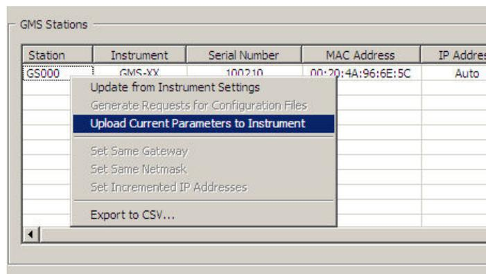
Figure 29. Upload parameters to the instrument
