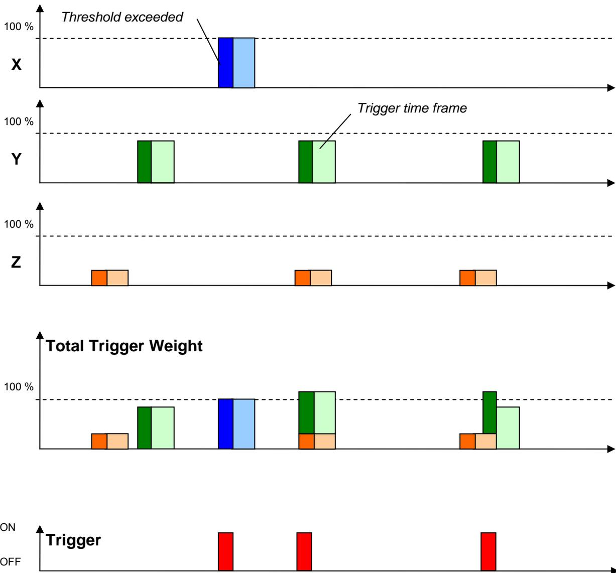
Figure 36. Overview of trigger weight and trigger time frame
