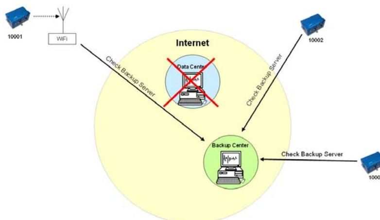
Figure 17. Connection to backup server in case connection to main server fails
