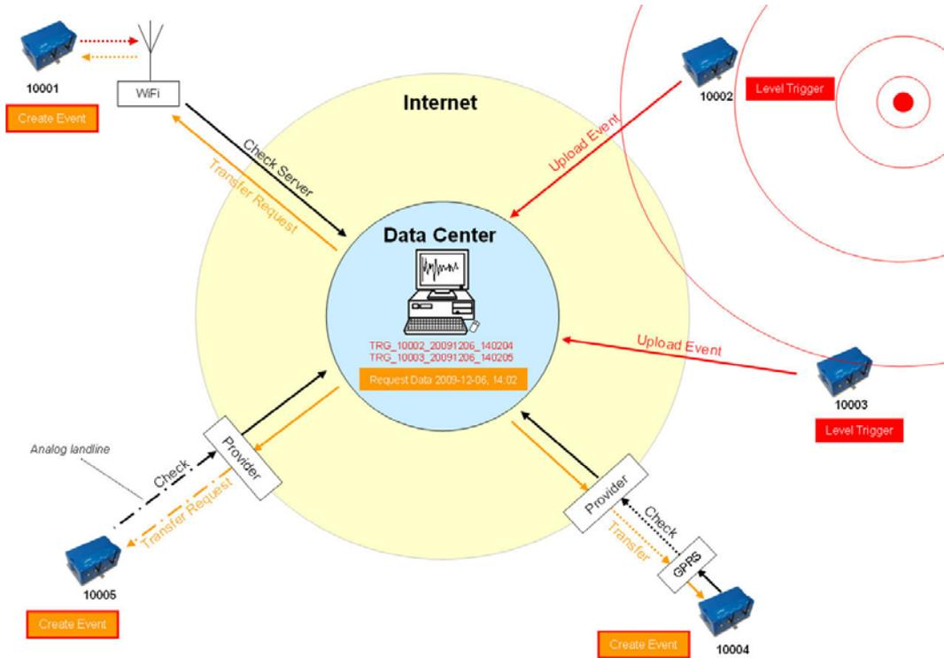
Figure 14. Upload of seismic events and download of requests from the server
