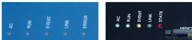
Figure 6. Visual indicators on the cover (left) and inside the instrument (right)
