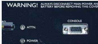
Figure 5. Internal RS-232 connector for the console
