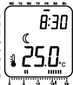
The Digital Thermostat is a weekly programmable thermostat, with 7 day/24 hour programs that can be set as required. For each hour you can set the Digital Thermostat so that either the CT (COMFORT) or ET (EVENING) temperature mode operates. The Digital Thermostat comes with a preinstalled program that will accommodate many users' requirements
